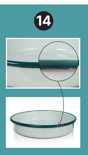
At cookware enamelling by manual dipping and the rim is in different colour comparing to external surface of the cookware item in one stage of the process an operator wipes off the excess of enamel from the rim after dipping. In a later stage of the process during drying enamel could additionally flow onto the rim surface and be visible after firing in the area where it has not been completely wiped so the rim remains in the colour of external enamel along the edge.
